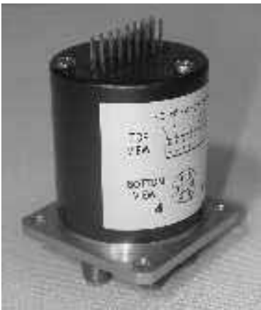
This Subminiature SPnT has been improved for automatic test benches where very low RF leakage is needed.
