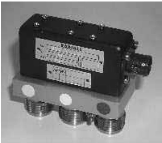
This SPDT with HN coaxial connectors and MILC38999 circular connectors for L band airborne applications.
